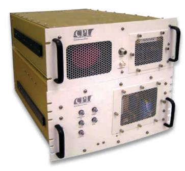
X-Band coupled cavity traveling wave tube transmitter with solid state pre-amplifier. Features a series of resonant high voltage power supply with dual depressed collector stages.
